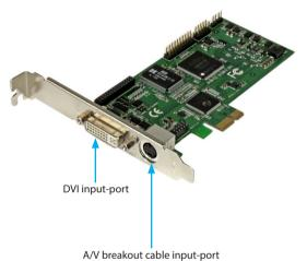
(For component, S-Video, and composite video input + RCA audio input)
